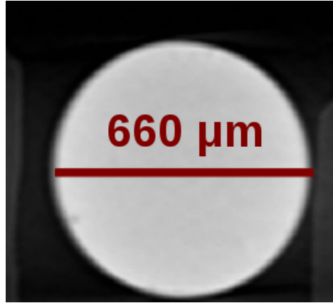
Figure 2.7 CT reconstruction of glass bead. Actual bead diameter is 660.4 \mu\text{m} .
